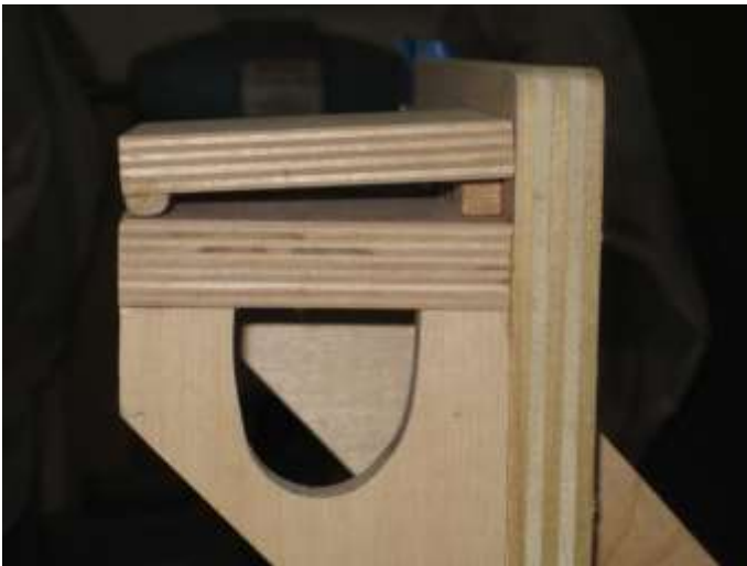
Figure 12: Bending Test Rig
