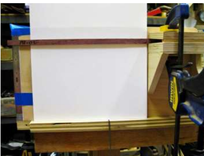
Figure 13: Bending Test Rig with Unloaded and Loaded Specimen
