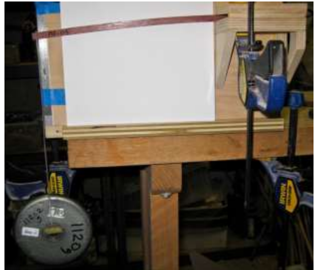
Figure 13: Bending Test Rig with Unloaded and Loaded Specimen
